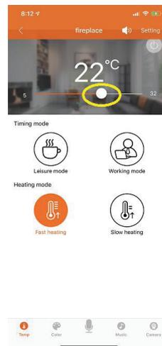
2) Lower the temperature: click Temp in the menu at the bottom of the APP, enter the temperature control interface, and drag the cursor from 5-32 to lower the temperature setting, with the lowest adjustable to 5 ° c;
