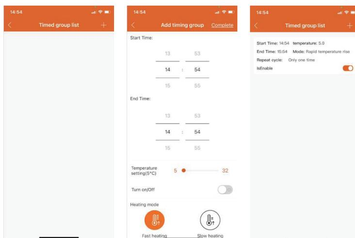
D) During the execution of the Work mode, the setting of manual debugging will be given priority to when the temperature is manually adjusted, and the Work mode will be canceled automatically. If you want to continue to execute the Work mode set in advance, please remember to re-execute the Work mode
